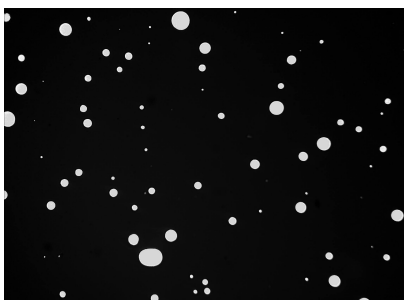
6.40 Concentrations of polypropylene in the base bitumen (0.5‰ by weight of aggregate).
