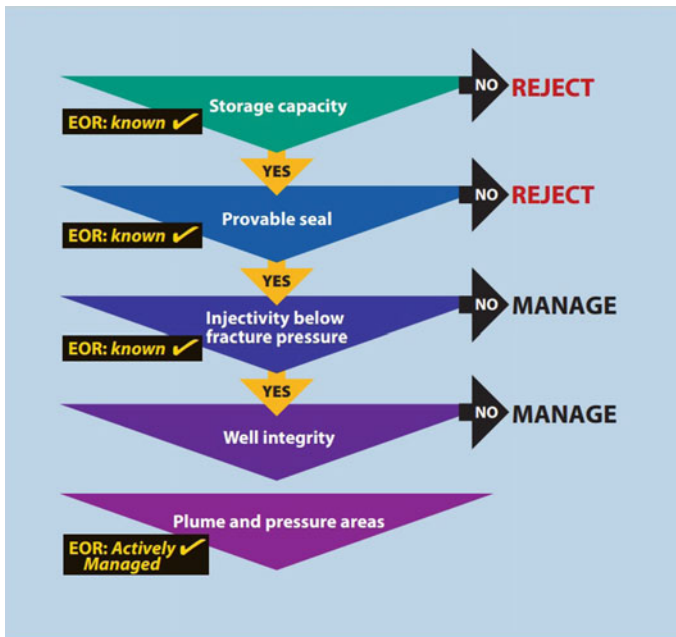
Fig. 6.2 Representation of the characterization and monitoring system for considering CO 2 storage in EOR. This also shows the criteria to accept or reject a storage proposal in EOR field (Hill et al. 2013)
