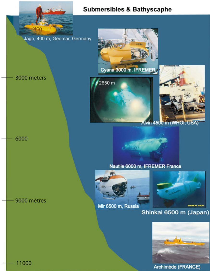
Fig. 3.2 Manned submersibles used for scientific exploration and their depth capabilities
