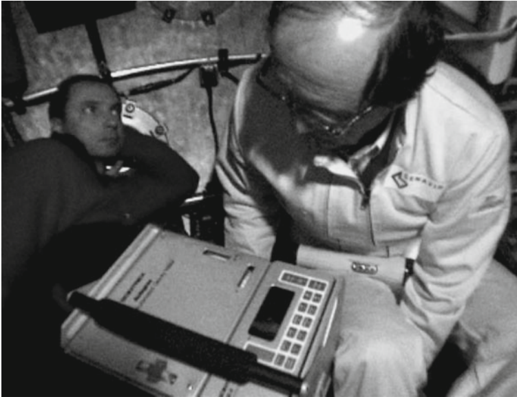
Fig. 9.17 The Nautilie dove on the Pitcairn hotspot's most eastern limit to measure the gravity anomalies at 3500–3700 m depth, at a distance from the base of the major volcanic edifices. Here we see the submersible's Pilot Justiniano (lying back) and Jacques Dubois (chief scientist) handling the gravimeter during dive. (Photo courtesy IFREMER, POLYNAUT cruise 1999, Nautilie dive PN07)
