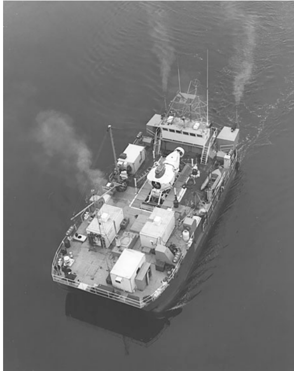
Fig. 7.14 The catamaran Lulu operated by Woods Hole Oceanographic Institution (USA). Aerial view of the support ship Lulu with its submersible Alvin hoisted up on deck. (Photo courtesy of WHOI Archives)
