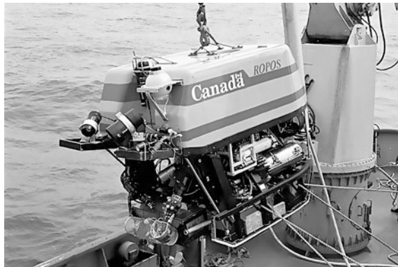
Fig. 3.5 Canadian remotely operated vehicle (ROV) called Ropos (Photo courtesy of S. Scott)
