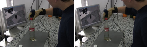
Fig. 19 Human demonstration of bottle opening task in sensory environment and simulation environment.
