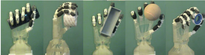
(b) Synthesized grasps with the DEXMART Hand.
