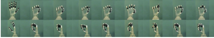
(a) First postural synergy. (b) Second postural synergy. (c) Third postural synergy.
