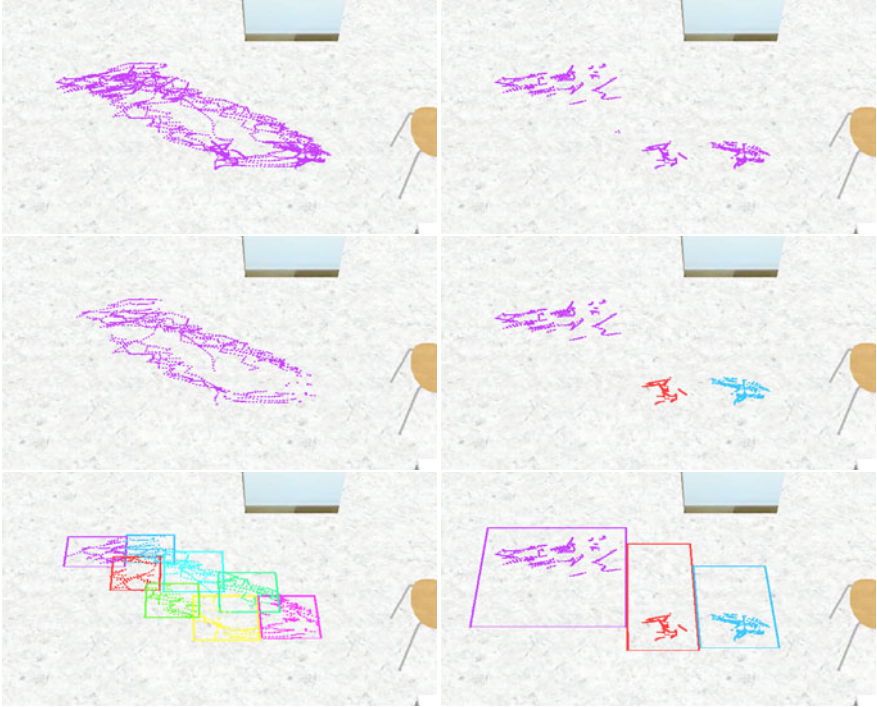
Fig. 36 Exemplary f_{feat_{self-pose}} generation: demonstration data (top left), filtered standing (top right), filtered walking (middle left), DBScan stationary clusters (middle right), k-means transition clusters and limits (bottom left) and final, merged region categories after BSP (bottom right).
