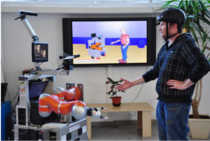
Fig. 1 The Jido robot interacting with a human. The robot model of the scene is displayed on the wall-screen. The Kinect monitors the human kinematics and the human gaze is perceived using a motion capture system. Robot motions take the human into account at planning and execution level.
