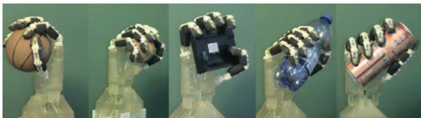
Fig. 23 Reproduced power grasps from the reference set of postures using the first three synergies.
