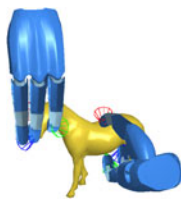
Fig. 8 An example of double grasp computed for right and left SAHs with friction cones displayed in colors.
