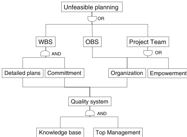
Fig. 14.1 Example of fault tree analysis
