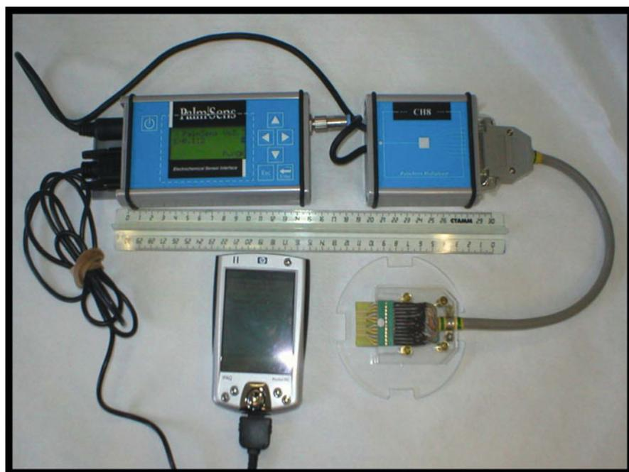
Fig. 2 Miniaturized electrochemical sensing device
