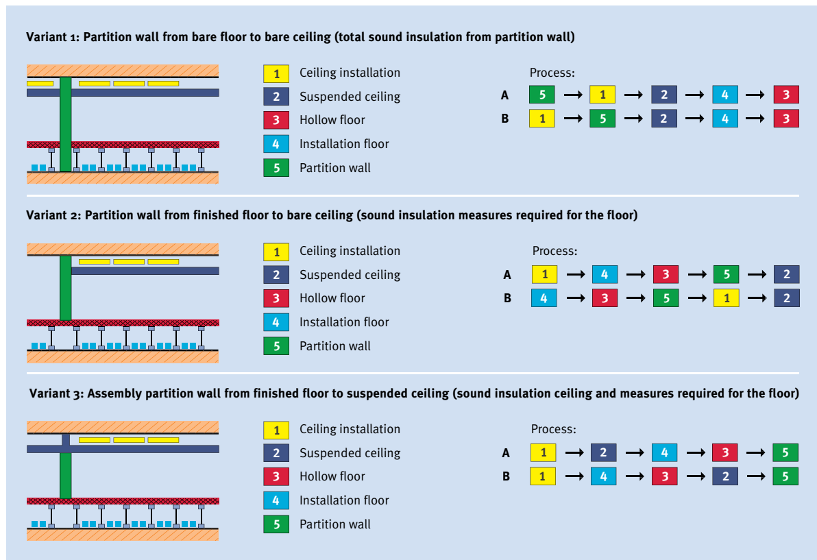
Fig. 3-71 Process varieties depending on partition wall structure
