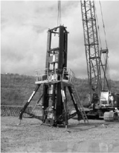
Figure 7.20 Picture of a Statnamic vertical load test (3 MN maximum load).
