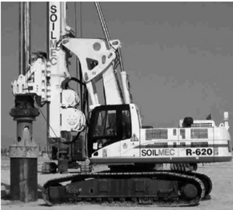
Figure 2.12 Temporary steel casing following the drilling tool.
