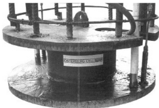
Figure 7.14 The Osterberg cell.
