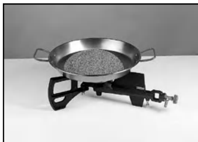
Figure 1.3. The frying pan method, also known as the frying stove method (CONTROLAB)
