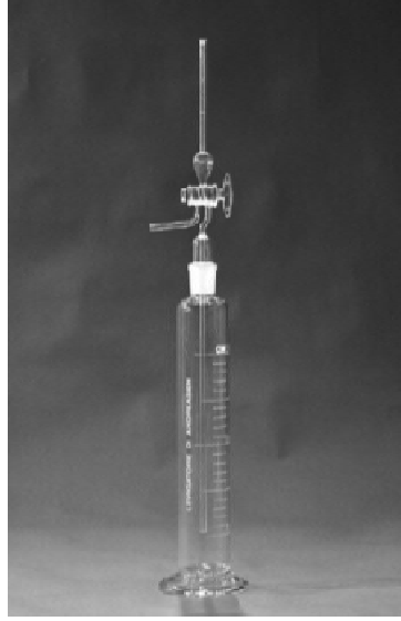
Figure 2.9. Diagram of an Andreasen pipette (NF X31-107), (CONTROLAB)
