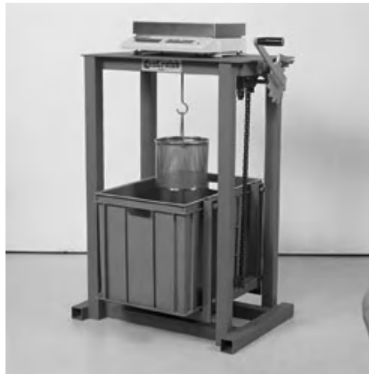
Figure 1.7. Built for hydrostatic weighing (CONTROLAB)
