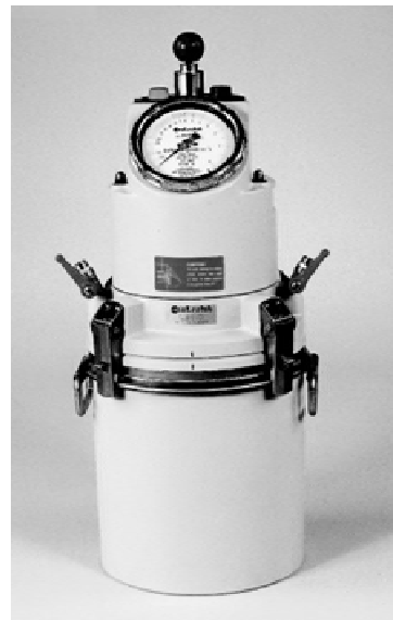
Figure 5.28. Sketch and photo of a concrete aerometer (CONTROLAB)
