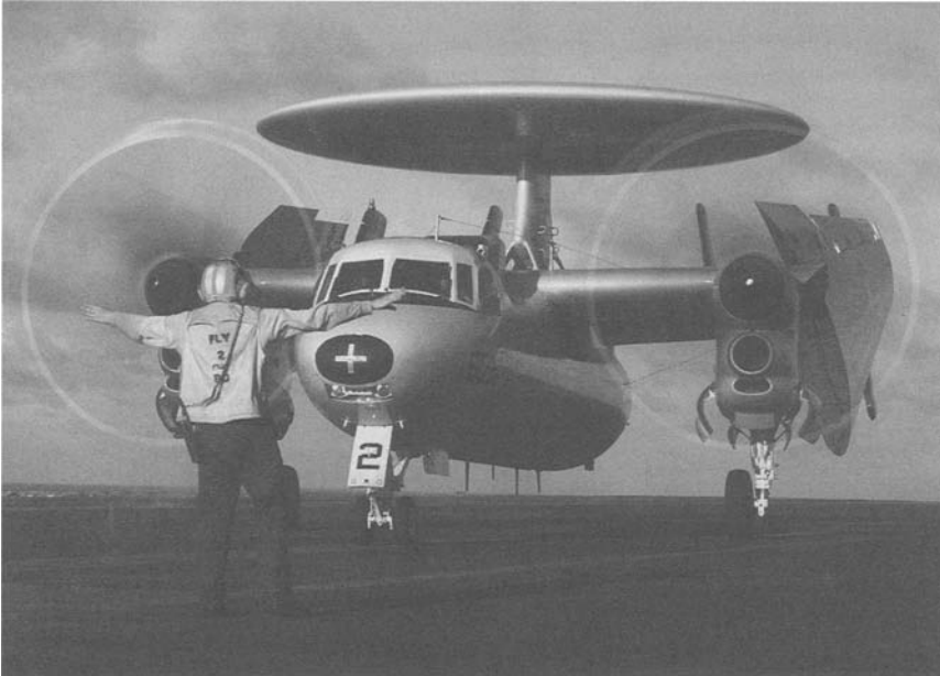
Figure 10.8. Hawkeye on the deck of an aircraft carrier. Note how its wings fold to save space in the cramped carrier. The folded wings accentuate the large area of the radome. US Navy photo.
