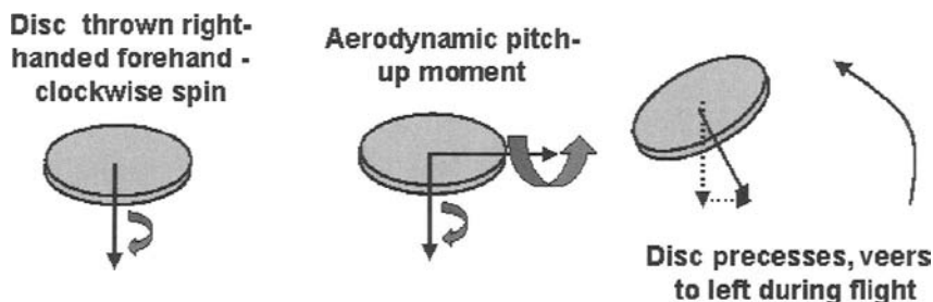
Figure 8.3. Schematic of the behavior of an object with pitch-up moment.
