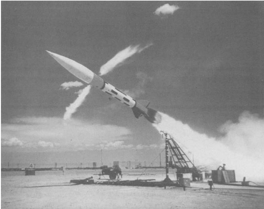
Figure 4.10. Honest John rocket leaving its launch rail. Bright plumes from just aft of the nose are two spin-up rockets. Photo: US Army Redstone Arsenal.
