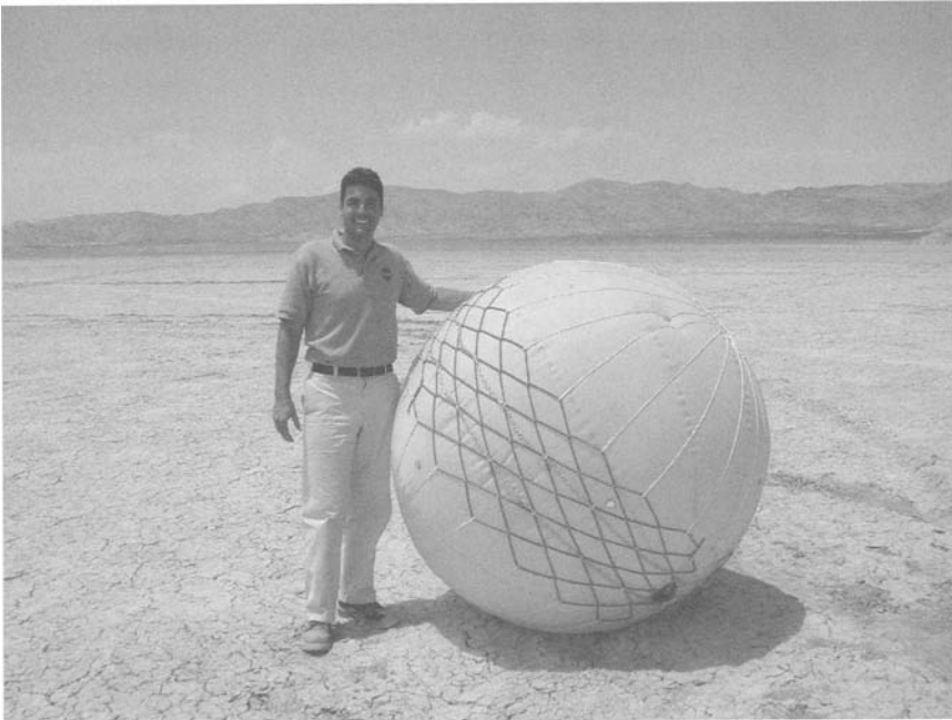
Figure 3.11. Engineer Alberto Behar with a Tumbleweed rover prototype in the Mohave desert. Note the diamond pattern of a web of cords intended to provide both abrasion resistance and traction, and a preferred roll axis via larger moment of inertia. Image used courtesy of NASA/JPL/Behar.
