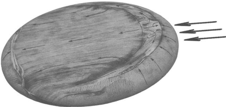
Figure 8.6. Perspective view of fluorescent paint flow. Notice how the surface flow diverges behind the leading edge, where the separation bubble reattaches. Figure by Potts and Crowther; used with permission.
