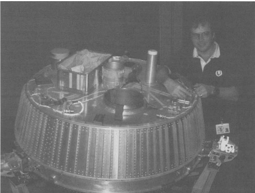
Figure 7.11. The Huygens SM2 model with the author at the European Space Operations Centre ESOC in Darmstadt, Germany, just a few days after the real probe arrived on Titan, 1.5 billion kilometers away. The large rectangular box on the top surface is the main parachute container.
