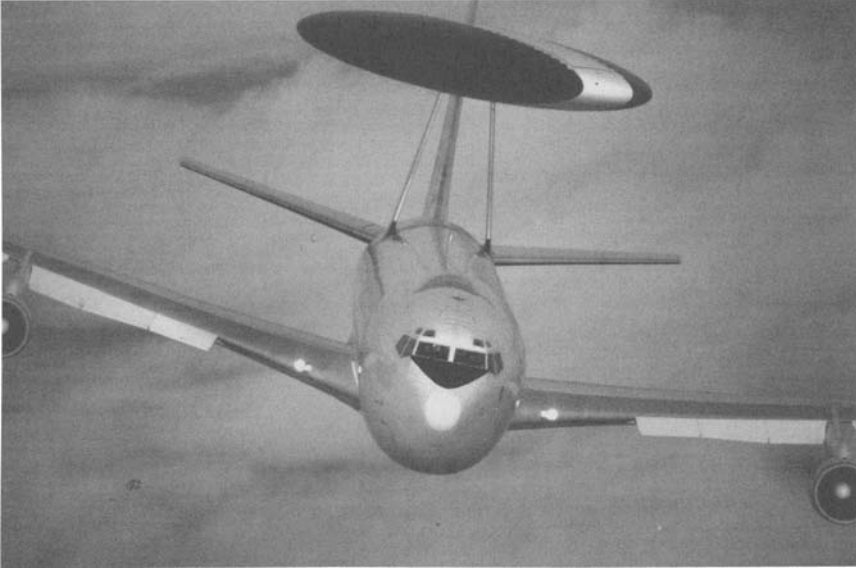
Figure 10.12. Head-on view of the E-3 with its massive radome. Note that the support structure uses two struts to provide adequate stiffness. This arrangement may also minimize wake effects on the tailfin. NATO photograph.
