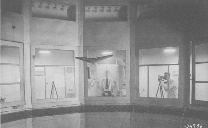
Figure 10.4. A model of the XB-47 free-flying in a larger spin tunnel at Langley in 1945. NASA Image EL-2000-00235.
