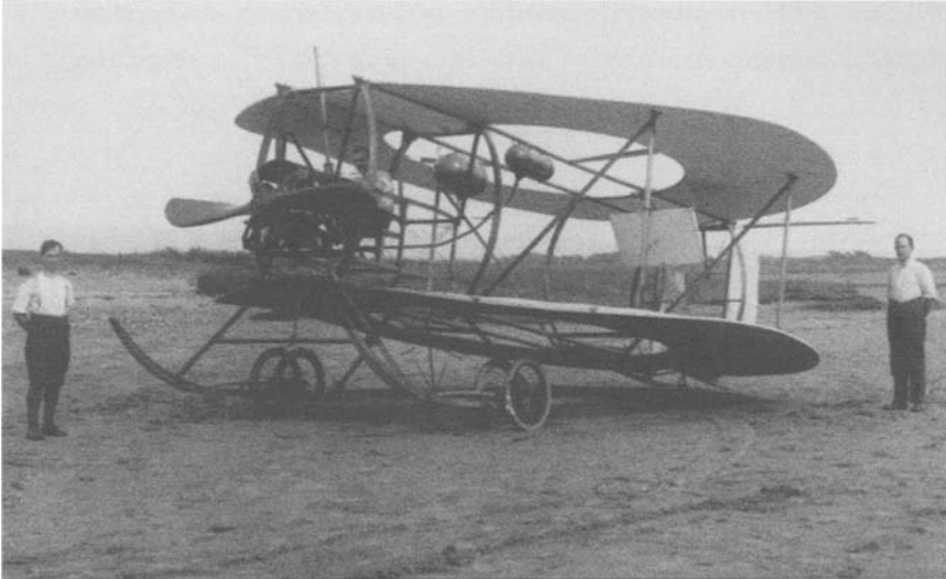
Figure 10.2. Lee-Richards powered biplane, with two annular wings and a conventional tail. From lantern slide in the collection of the Royal Aeronautical Society.
