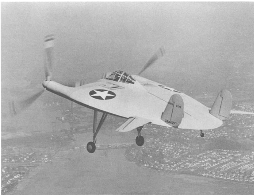
Figure 10.6. Vought V-173 in flight. Notice the three-bladed propellers and the tall undercarriage, both to hold the aircraft at high angle of attack for lift, and to keep the propeller tips from striking the ground! Photo courtesy of Vought Aircraft Industries, Inc.
