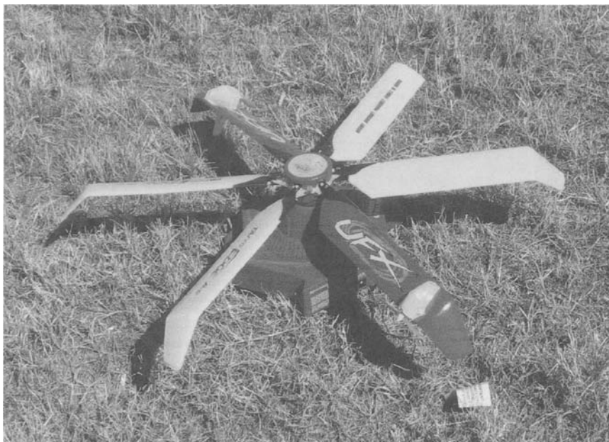
Figure 10.18. The Taiyo Edge on the author’s lawn. Small propellers are driven on two of the six rotor blades.
