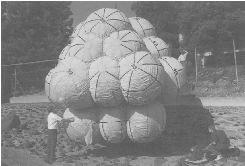
Figure 3.8. The Mars Pathfinder lander in a ground test, encased in its cluster of airbags. NASA image GPN-2000-000484.
