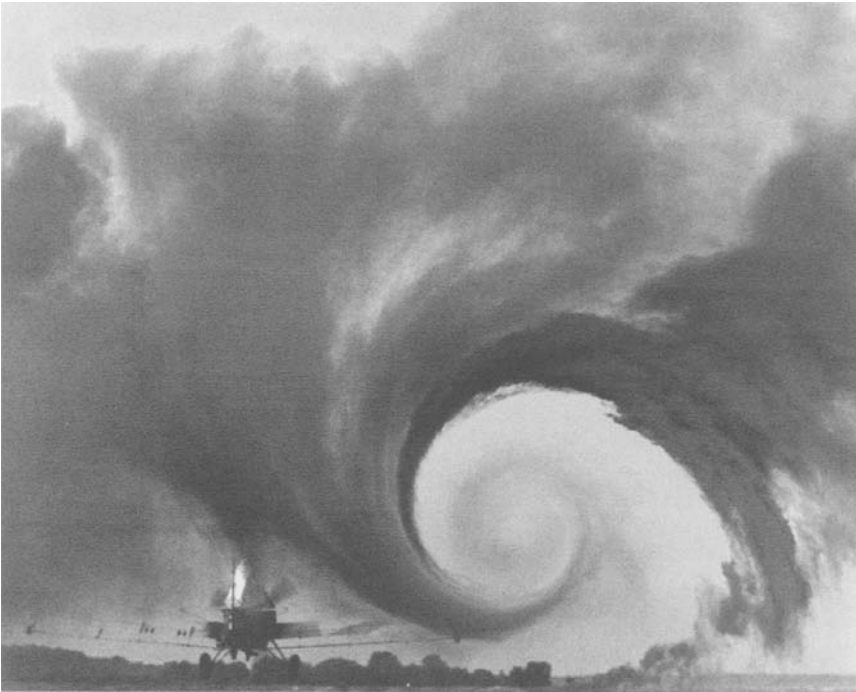
Figure 10.1. The strong wingtip vortex as air spills from under the wing visualized by smoke in a test by NASA Langley at Wallops Island. NASA Image EL-1996-00130.
