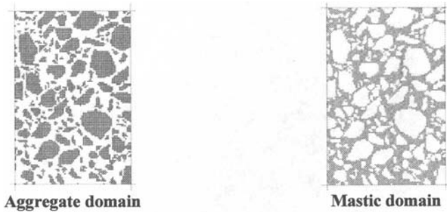
b) Discrete elements of the aggregate and mastic phase with 0% air void content
