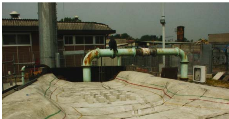
Figure 9. Upstream part of the physical model where the model city has been located (aligned city layout)
