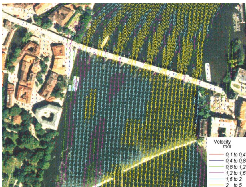
Figure 9. Velocity field close to the Charles bridge area
