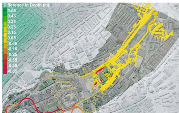
Figure 8. Example output from 2D hydrodynamic model. Difference in depth (m) before and after proposed development for 100 year return period flood (plus 20% for sensitivity)
