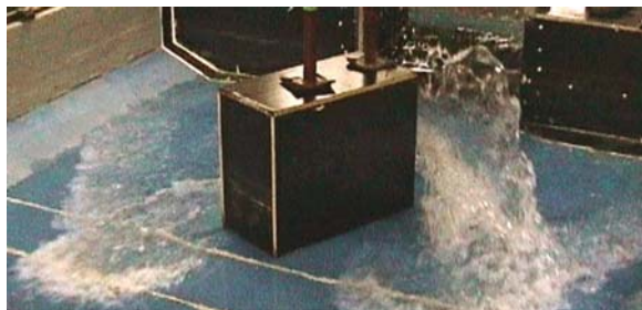
Figure 1. 3D surge against the building in laboratory experiment
