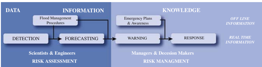
Figure 1. Flood warning as a process
