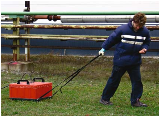
Figure 2. GPR measurement (200 MHz antenna)
