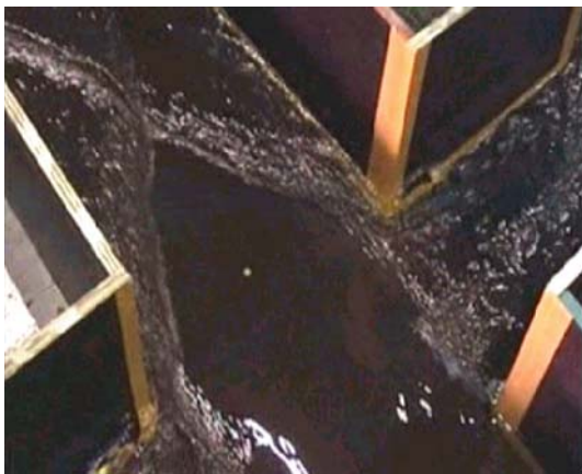
Figure 4. Cross waves at an idealised crossroad in the laboratory (UCL)
