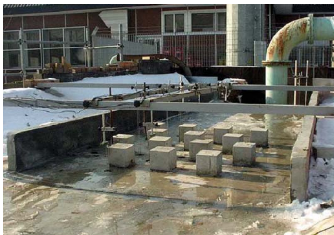
Figure 10. The simplified morphology version of the valley with staggered city layout
