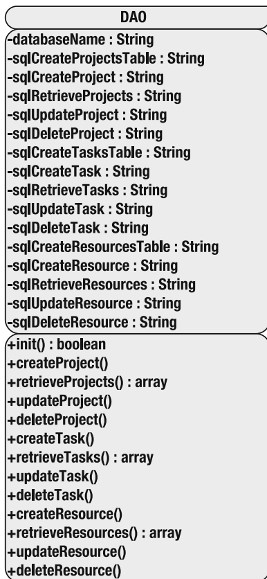
Figure 4-4. UML class diagram of the DAO class
