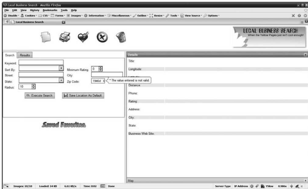
Figure 8-6. An error resulting from entering a letter in the Zip Code field
