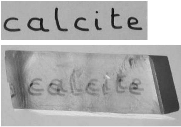
Figure 1.6. An example of the optical effect when viewing an object through “Iceland Spar” crystal. (Photograph courtesy Joanna Edkins)
