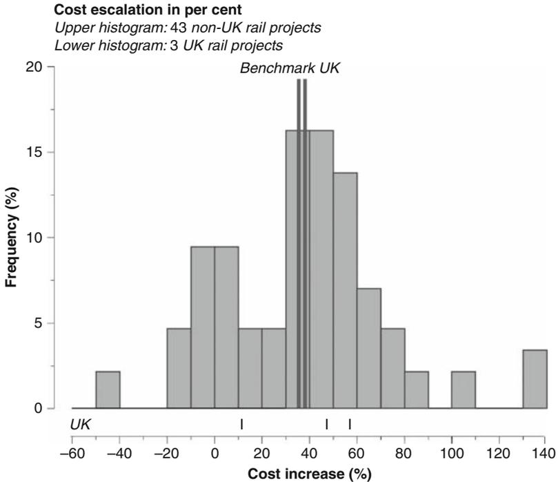
*Figure 8.1* Inaccuracy of construction cost forecasts for rail projects in reference class. Average cost increase is indicated for non-UK and UK projects separately. Constant prices
