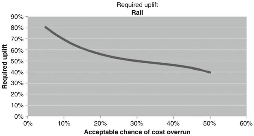
Figure 8.2 Required adjustments to cost estimates for UK rail projects as function of the maximum acceptable level of risk for cost overrun. Constant prices
