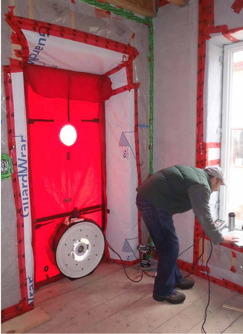
A blower door is used to depressurize the building to test for airtightness.
