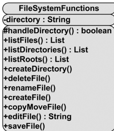
Figure 6-17. UML class diagram for the FileSystemFunctions class
