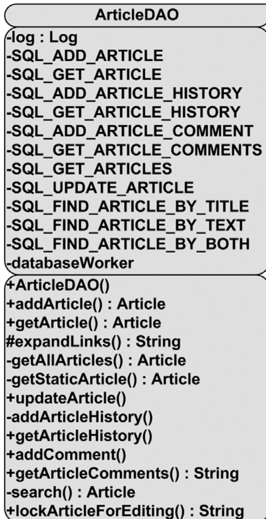
Figure 5-19. ArticleDAO class UML diagram
