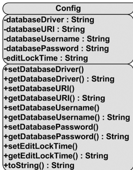
Figure 5-11. Config class UML diagram
