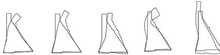
Figure 2. The first five mode diagrams of dam.
