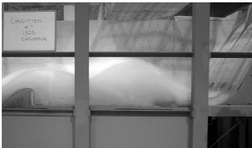
FIGURE 11-1. 1:36 Scale Section Model of Bluestone Lake Dam, New River, West Virginia. Courtesy of U.S. Army Corps of Engineers.
