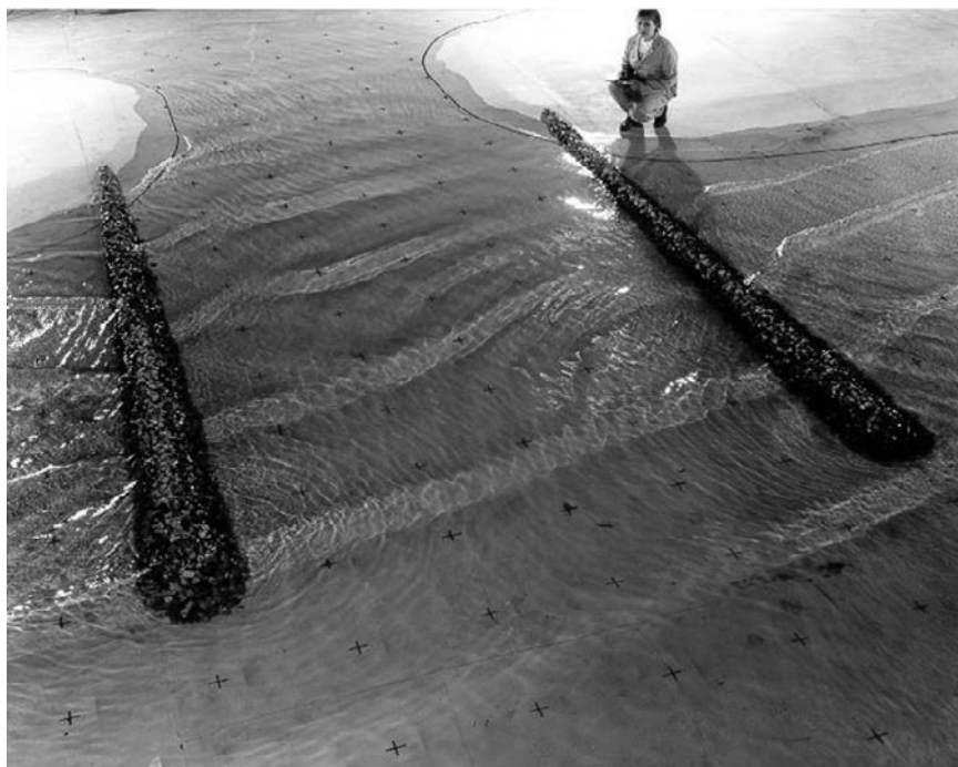
FIGURE 11-3. Jetties under Study on Idealized Inlet Research Study at WES. Courtesy of U.S. Army Corps of Engineers.
