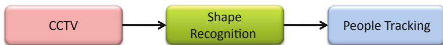
Fig. 9.1 A simple example for smart surveillance. A single data source (CCTV) is the input for a single data processing stage—in this case, a tool to automatically detect human shapes (e.g., in a parking lot). Ultimately, this tool allows the system to track people in a parking lot, highlighting them to a human operator and keeping statistics on movements in the parking lot over time
