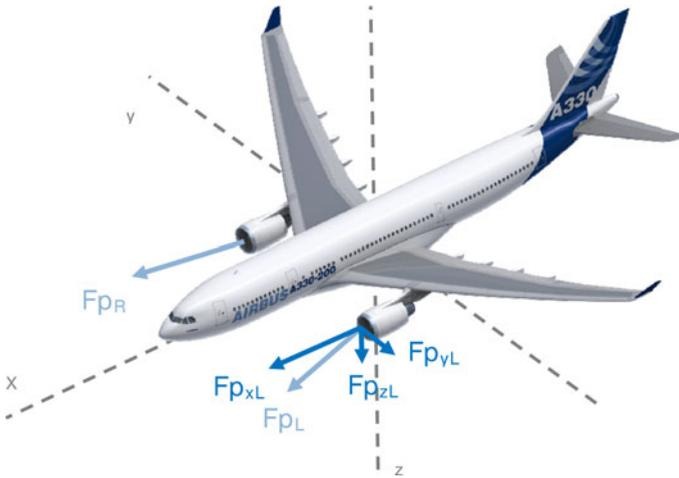
Fig. 2.9 Representation of engine thrust forces
