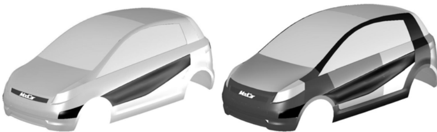
Fig. 8.9 Outer surface of the ModCar (hatchback) and the partition strategy
