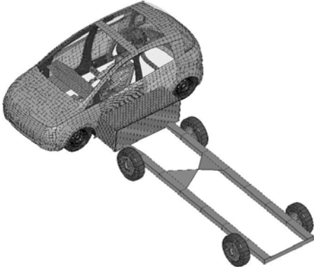
Fig. 8.16 Load case configuration side impact in accordance with Euro-NCAP
