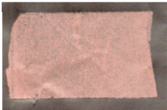
Figure 3. Adhesion (Scotch tape test) of PVDF/LBG1025 coating showing poor adhesion of graphite to copper current collector.
