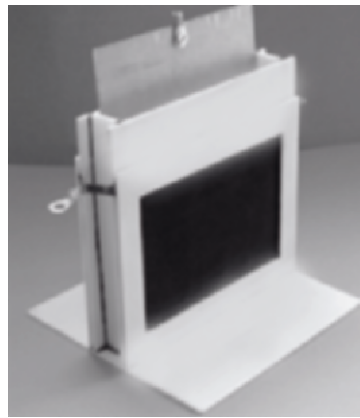
Figure 6. Experimental mechanically rechargeable Mg-air cell.
