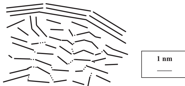
Figure 6. Sketch of the cross-section of a carbon fiber coated by pyrocarbon, taking into account the HRTEM image analysis data.
