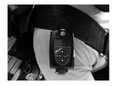
Figure 3. Audio dosimeter (Model: The Edge5— Quest/3M) installed in the participant's auditory zone.
