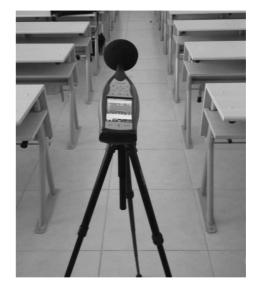
Figure 1. Hand-held analyzer type 2250 during measurement.
