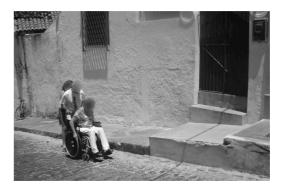
Figure 1. Excessive height between streets and sidewalk and steps along sidewalks compelling users to move along the roads. Source: author's collection (2008).
