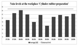
Graph 4. Noise levels at the workplace 'Cylinder rubber preparation'.
