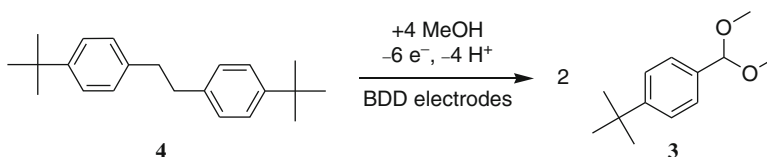
Fig. 5.8 Bond cleavage in 1,2-DPTE in the synthesis of p - tert -butylbenzaldehyde dimethyl acetal (3). Reagents and conditions: BDDE, 2% 1,2-DPTE, 0.5% H 2 SO 4 (96%), MeOH, 3.4 A dm -2 , 54°C, 8 F mol -1 ; yield = 47% (3)
