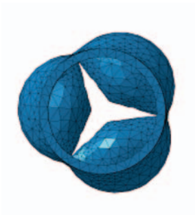
Figure 1.7. Top view of a mesh of the aorta root with the three leaflets of the aortic valve and the Valsalva sinuses (from T. Cherigui).
