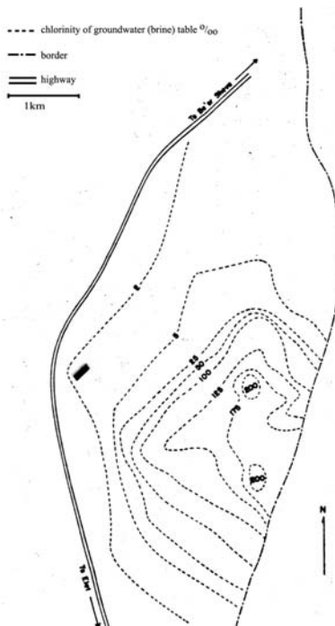
Fig. 8.2.3-4 Map showing changes in chlorinity (mg kg -1 ) of groundwater across Yotvata Sabkha (after Amiel and Friedman, 1971).
