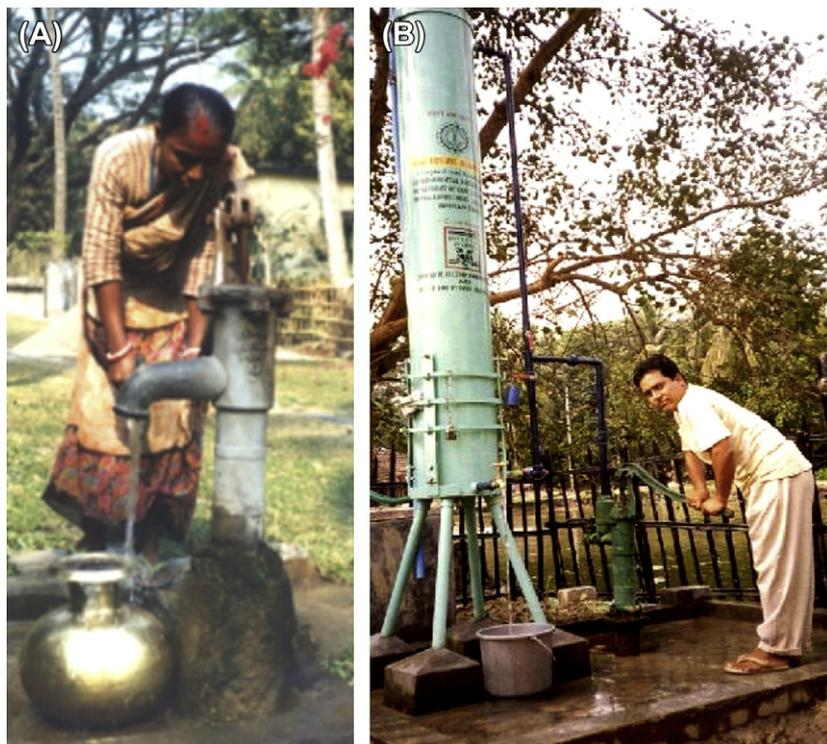
**FIGURE 13-1** (A) Conventional method of water collection and (B) an arsenic-removal unit showing the method of water collection. (For color version of this figure, the reader is referred to the online version of this book.)
