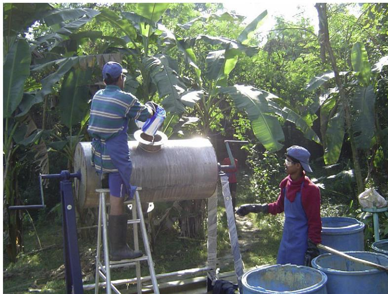
**FIGURE 13-6** A regeneration reactor being operated at the central regeneration facility at N 24 Parganas, West Bengal. (For color version of this figure, the reader is referred to the online version of this book.)
