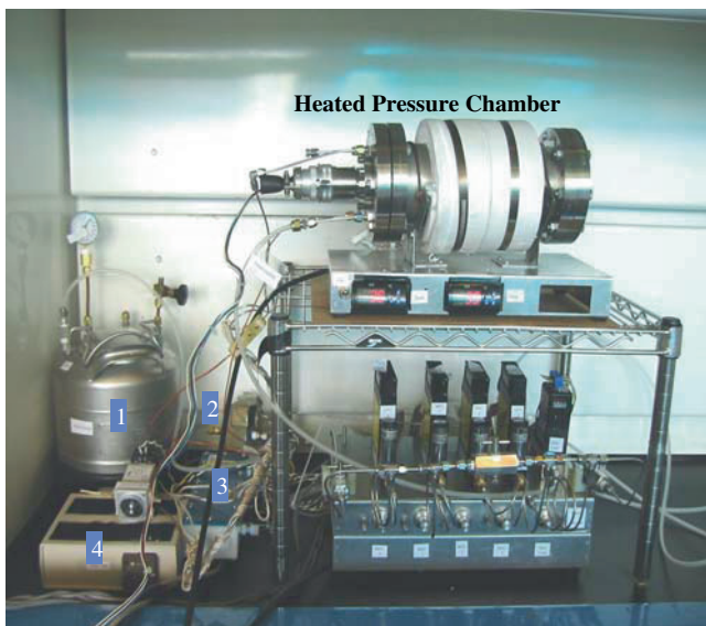
Fig. 1.10 SSTUF apparatus illustrating chamber for evaluation of chemical sensors and arrays
