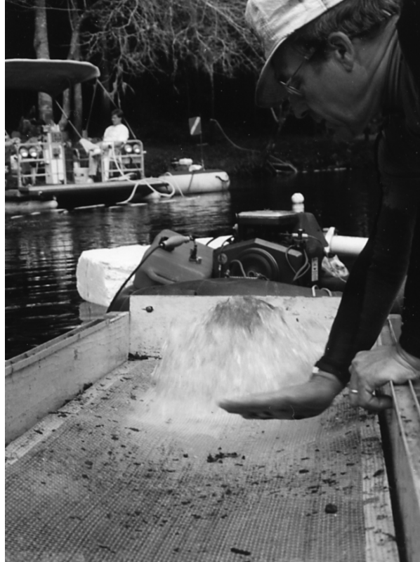
Figure 1.12 Screendeck operator monitors tailings delivered from dredge excavation. Colour version of this figure can be found in Appendix on page 553. Photo credit – Robin Brown.
