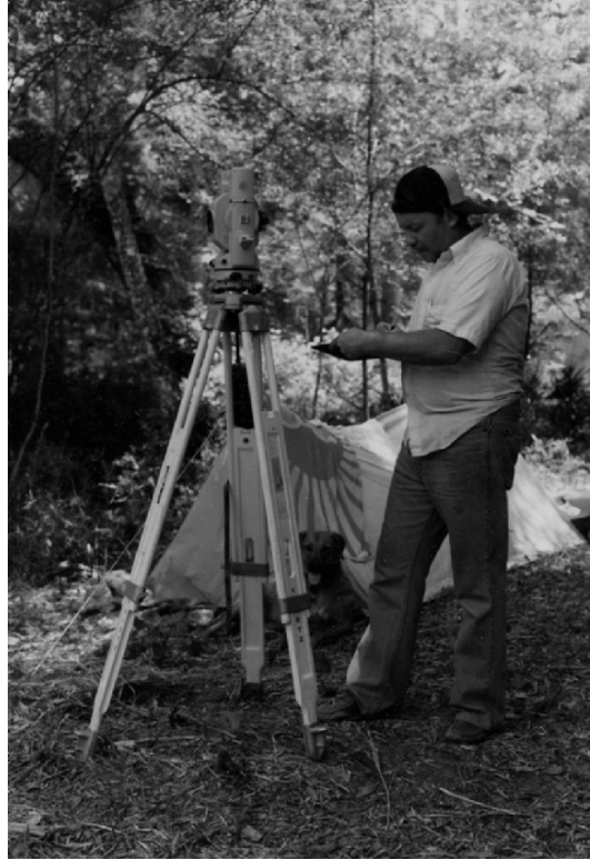
Figure 1.8 Surveyor shoots terrestrial elevation down to Page-Ladson Site river level datum. Colour version of this figure can be found in Appendix on page 553. Photo credit – Joseph M. Latvis.
