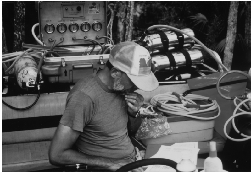
Figure 1.4 Surface supplied air control station showing monitoring/distribution instrumentation directly (behind divemaster), accumulator tanks (right), and high pressure backup cylinder (left). Colour version of this figure can be found in Appendix on page 553. Photo credit – Susan Verberg.
