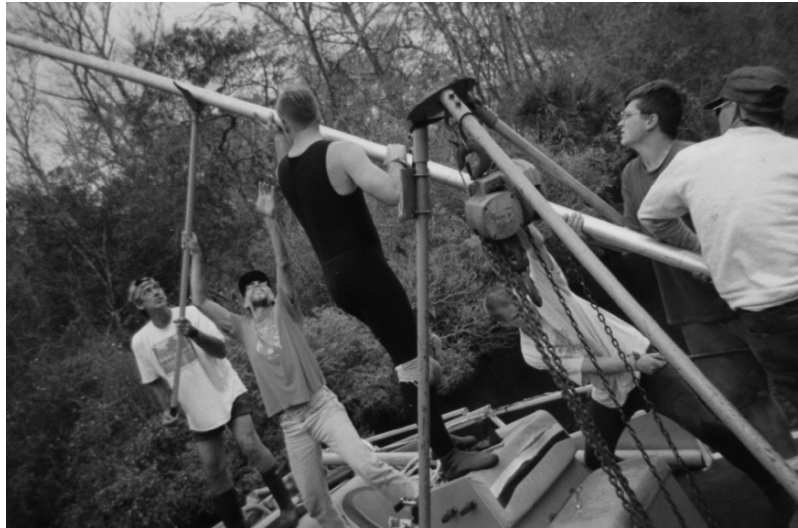
Figure 1.6 Note steel tripod with chain hoist for extracting coretube. Bottom sediment coring team hoists vibracore tube into position aboard operations barge. Colour version of this figure can be found in Appendix on page 553. Photo credit – Thadra Palmer Stanton.
