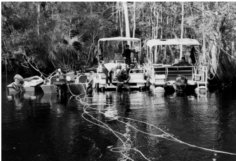
Figure 1.1 Note two sets of SSA hose lines supplied by the air control station on the diving operations barge emanating toward the right foreground, where two dive teams are simultaneously excavating two discrete units. Research vessel deployment at typical riverbank site: (right to left) diving support vessel, diving operations vessel, emergency evacuation vessel, and chase/communications vessel. Colour version of this figure can be found in Appendix on page 553. Photo credit – Susan Verberg.
