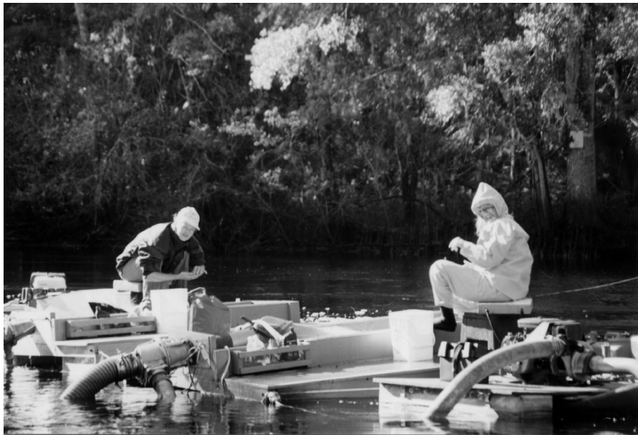
Figure 1.3 Typical screendeck barge deployment midriver: (right to left) 18-horsepower dredge pump (on separate flotation) powering 6-inch couplejet dredge mounted into screendeck barge. Mirror image arrangement powers 4-inch couplejet dredge on far left. Colour version of this figure can be found in Appendix on page 553. Photo credit – Krister Efverstrom.
