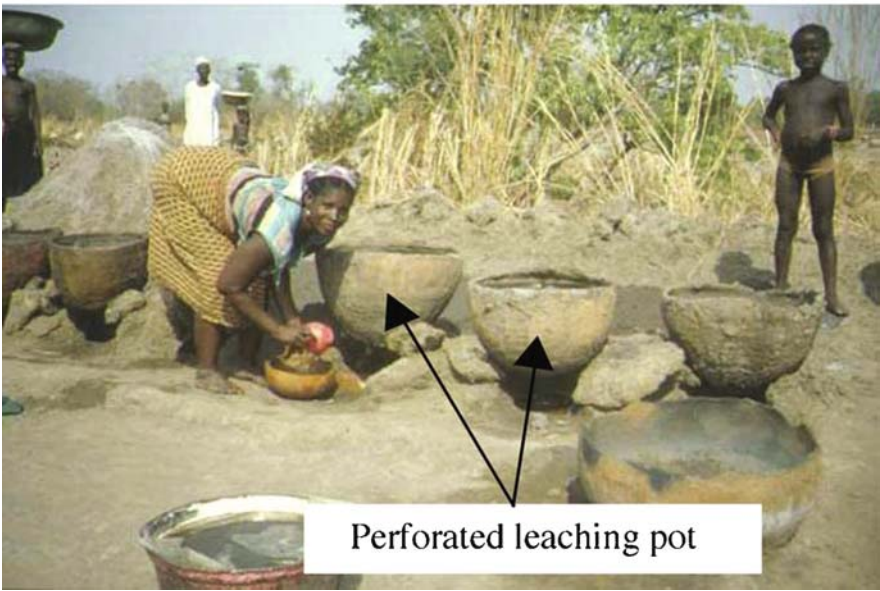
Fig. 10.25 Salt processing center at Ribi in Nasarawa state, showing boiling to dryness and crystallization of salts from the brine leachate. (Captured from Tijani and Loehnert, 2004)
