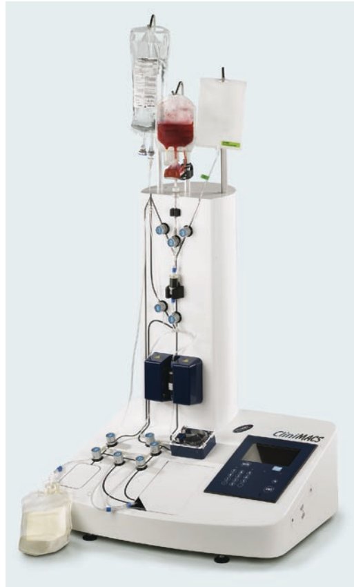
Fig. 8 CliniMACS® Plus Instrument. The CliniMACS System is an automated cell separation system for clinical-scale magnetic enrichment of target cells or depletion of unwanted cells in a closed and sterile system. For separation, a single-use tubing set, including a separation column, is attached to the CliniMACS Plus Instrument. Then the cell preparation bag containing the labeled cells is connected to the tubing set. After starting the separation program, the system automatically applies the cell sample to the separation column, performs a series of washing steps, and finally elutes the purified target cells. The CliniMACS® System components (Reagents, Tubing Sets, Instruments and PBS/EDTA Buffer) are manufactured and controlled under an ISO 13485 certified quality system. In Europe, the CliniMACS System components are available as CE-marked medical devices. In the USA, the CliniMACS System components including the CliniMACS Reagents are available for use only under an approved Investigational New Drug (IND) application or Investigational Device Exemption (IDE). CliniMACS® MicroBeads are for research use only and not for use in humans
