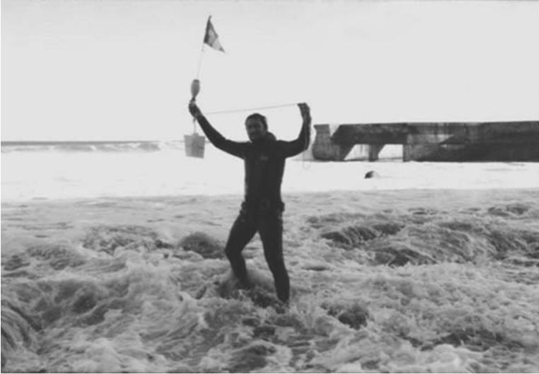
**FIGURE 15.2** Drogue with fins for sampling current below water surface.
