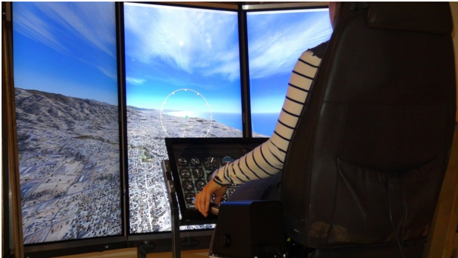
Fig. 1. Experimental setting with visual primary head-down display, and visual head-up drift display on the central screen
