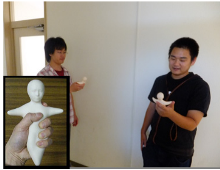
Fig. 1. Elfoid: cellular phone-type teleoperated android
