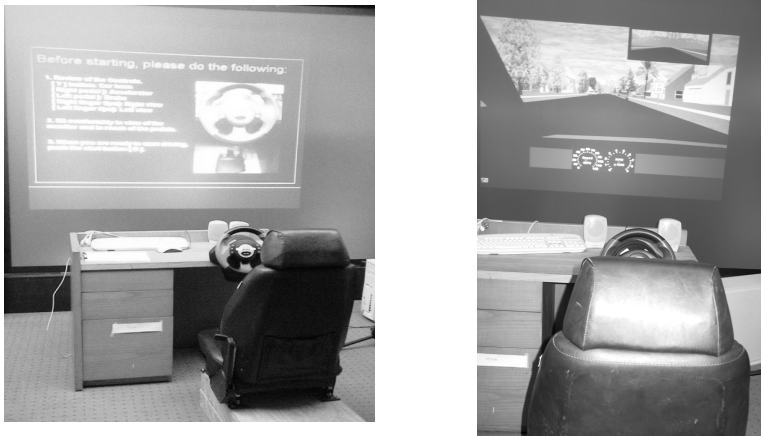
Fig. 1. STISIM Drive - Driving simulator. Setup Screen and random road scene depicted.
