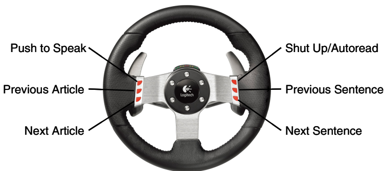
Fig. 2. Steering wheel buttons layout
