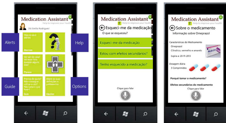
Fig. 5. Graphical user interface of Medication Assistant depicting the main screen, advice on forgetting the intake of medicine and detailed information of medication
