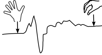
Fig. 8. The gesture parsing by seeking big difference in hand movements
