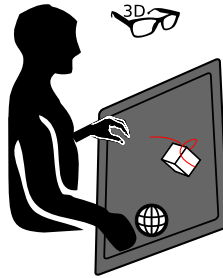
Fig. 1. The manipulation of the gestures on and above the table, using 2D and 3D virtual objects and captured via 3D sensors
