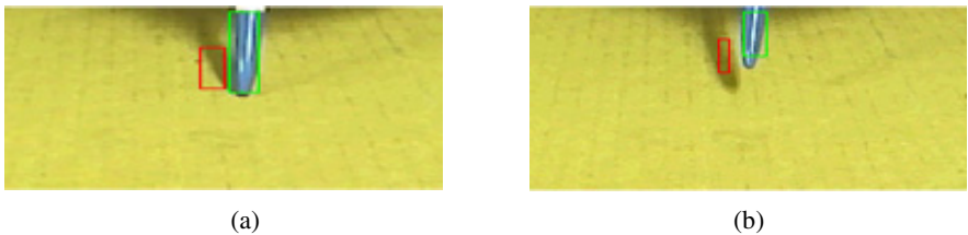
Fig. 10. The correct detection result: (a) the pen touching the tablet; (b) the pen leaving the tablet under its tilt angles between -16^\circ and 16^\circ for m = 5
