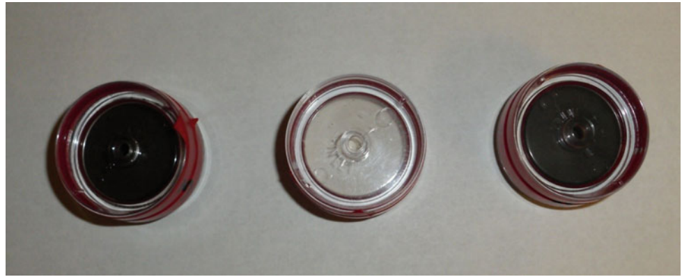
Fig. 2 Filters with particulate matter collected from non-mining ( middle ) and mining ( left and right ) residential areas
