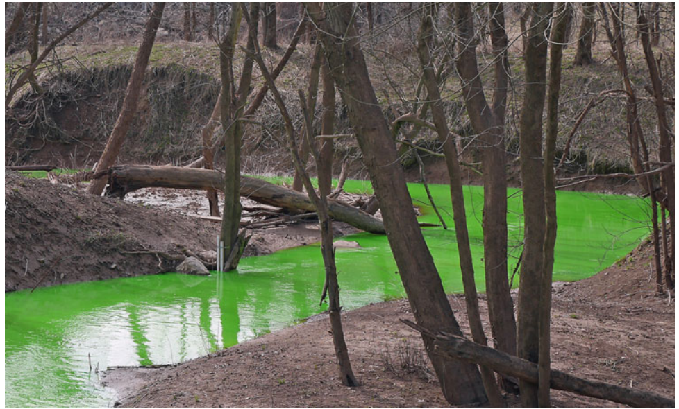
Fig. 1 Photograph showing the tracer dye fluorescein sodium in a sinking stream. Recovery concentrations are generally kept below the visual threshold (about 100 ppb), and the limit of detection is less than 0.1 ppb
