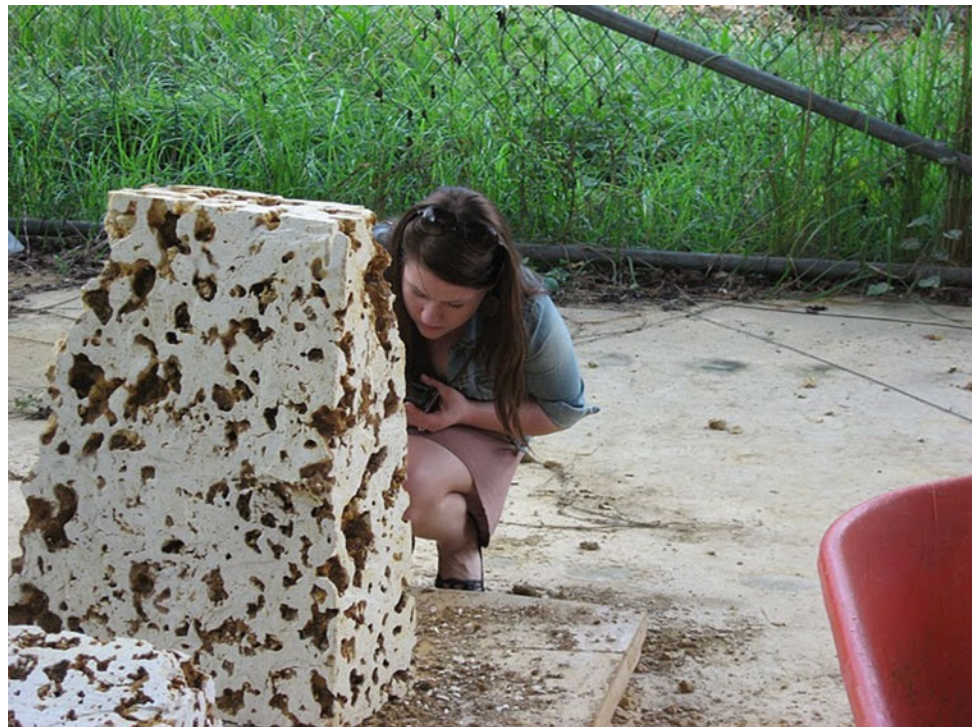
Fig. 4 Block of vuggy limestone from the north coast karst aquifer of Puerto Rico
