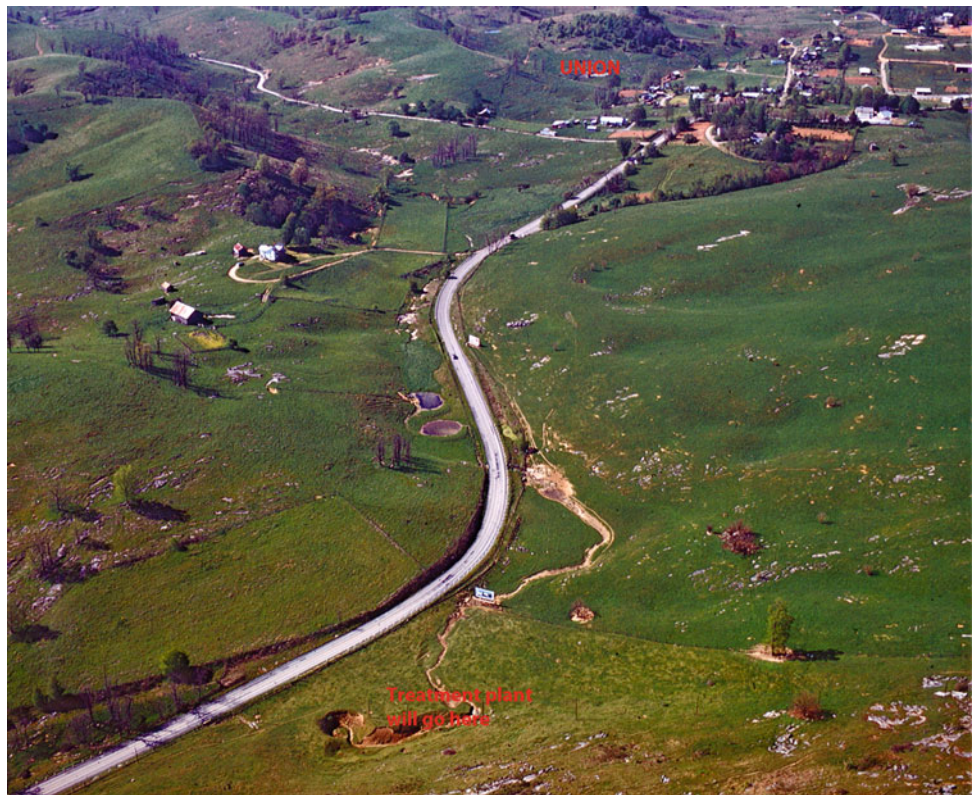
Fig. 5 Aerial photograph showing the location of the new (1973) sewage treatment plant for the town of Union. The treated effluent flows into a sinkhole, and the plant is subject to flooding
