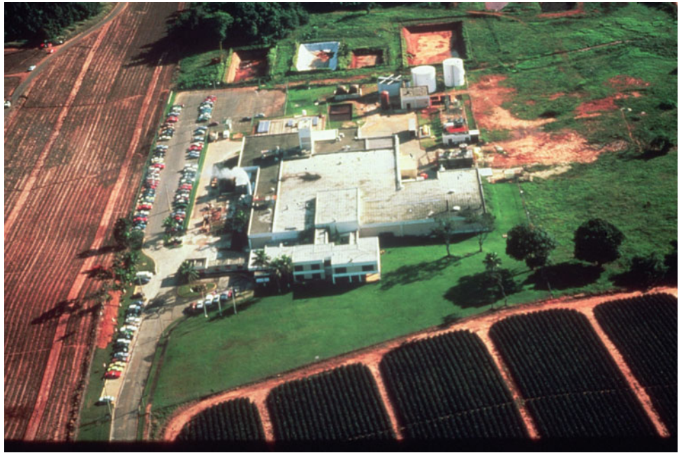
Fig. 7 Aerial view of the RCA del Caribe Superfund Site, Barceloneta, P.R. where small and large spills from tanker trucks occurred during normal operations. Note the four liquid hazardous waste surface impoundments at the top of the photo and the sinkhole evident in the left-most surface impoundment
