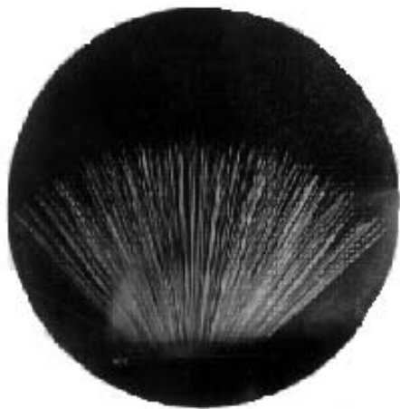
Fig. 1.1. Tracks of alpha particles in a Wilson cloud chamber. The scale is about 1:2. From Meitner and Freitag (1926)
