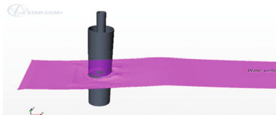
Fig. 5.19 Simulation of inner cylinder with perforated outer cylinder (Chandrasekaran et al. 2014)
