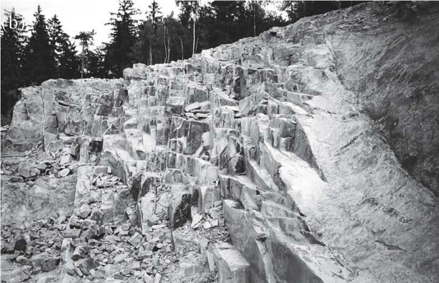
Fig. 2.69b. Joint bifurcation by sudden stress release. South Bohemian Pluton. The large block at right bifurcates towards left (note optical distortion)
