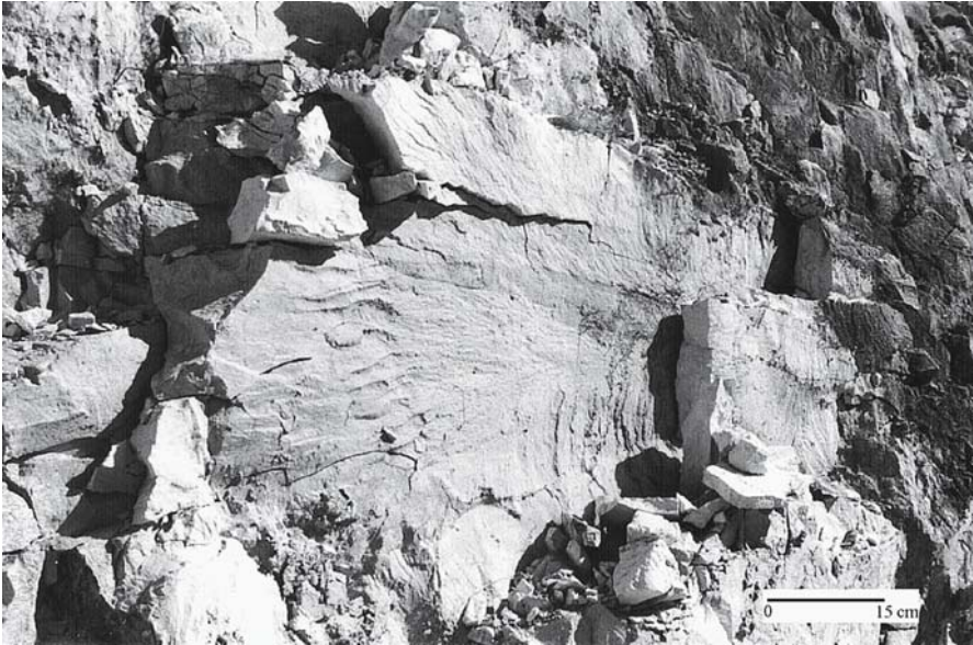
Fig. 2.42. Cusped hackles. A plume developed into right-stepping and left-stepping echelons at the upper and lower parts of the marking, respectively, but transformed laterally towards left into cusped-hackles, suggesting a lateral cracking under conditions of greater stress intensity. From an Upper Cretaceous chalk in south England (after Bahat 1991a)
