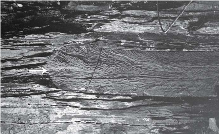
Fig. 6.1. An exact joint tip is shown by the sharp distal boundary (arrow) of the plume, for measuring joint lengths. Width of joint is 20 cm
