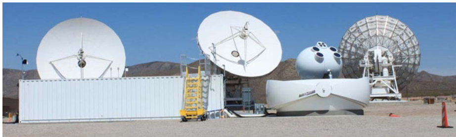
Fig. 3 The Lunar Lasercom Ground Terminal at site (White Sands, NM). The four smaller uplink telescopes can be seen grouped above the four 40 cm downlink telescopes
