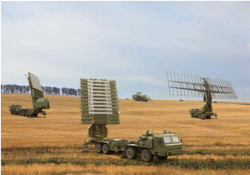
Fig. 10.10 The Nebo-M radar complex, comprising 3 radars in different bands (metric, deca-metric and centimetric, in terms of wavelength, or VHF, L and S/X, in terms of frequency) and a control station, performing sensor fusion [19, 23]
