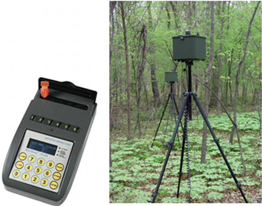
Fig. 12.1 Bio-seed ® hand-held, battery operated analyzer for in situ identification of bioagents-Left. Right, BAWS ® fixed, movable sensors for surveillance in linear formation
