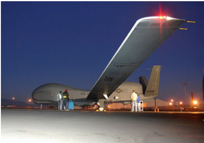
Fig. 12.2 Long-range (or “High Altitude Long Endurance”—HALE) huge UAVs, like the US Q-4 family, may carry sensors and assaying equipment to process samples in situ and transmit results by data link while on patrol
