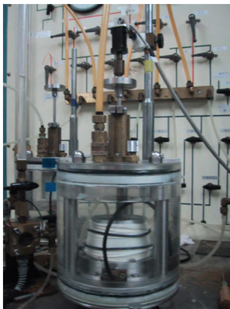
Fig. 4.6 Setup of the consolidation cell. (a) Sketch; (b) Photo
