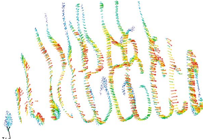
Fig. 48 Sample velocity vector field in different sections of the nasal airways
