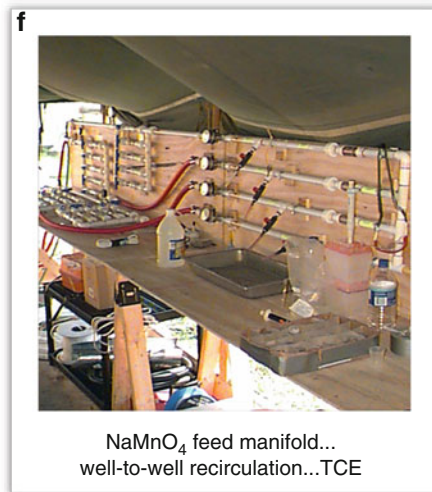
Figure 1.11. Photographs illustrating some of the conditions and infrastructure at sites where ISCO has been deployed for groundwater remediation. Image captions give oxidant used, delivery method, and target contaminants. Note: CB - chlorobenzene, MGP - manufactured gas plant.
