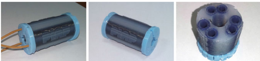
Fig. 1 Single module design. On the left module; on the right module cross-section, reinforced actuation chambers and central channel visible
