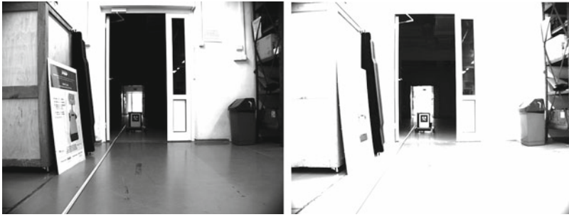
Fig. 9 Images taken during experiments. Left one shows picture taken with standard exposure control algorithm, right one with proposed one
