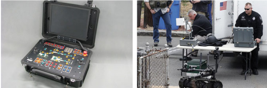
Fig. 2 Control console of PIAP Ibis robot and an example of complex way of mobile robot teleoperations. Sources http://antyterrorism.com , http://dailymail.co.uk
