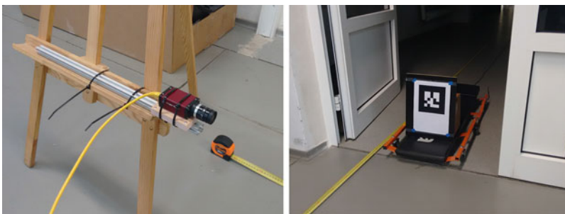
Fig. 8 Experimental setup. Left picture shows Manta G-282B camera, right shows marker used
