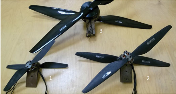
Fig. 3 Comparison of tested propulsion units 1 MN3110 + 10" prop., 2 MN4014 + 16" prop., 3 U8 Pro + 26" prop
