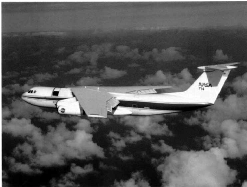
Figure 7.17. The Kuiper Airborne Astronomy (KAO) aircraft. Courtesy of NASA.
