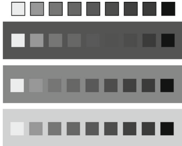
Fig. 3.6 A set of objects with reflectance factors typical of those found in a pedestrian's clothing ( top ), seen against three different road-surface backgrounds, in order of increasing luminance. With good road lighting most of the objects are seen in negative contrast (silhouette vision)
