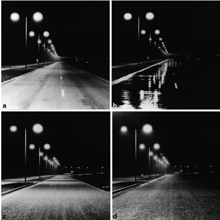
Fig. 2.2 The influence of road-surface reflectance on perceived brightness, with illuminances constant: a smooth dry surface; b smooth wet surface; c rough dry surface; d rough wet surface. (Van Bommel and De Boer 1980)
