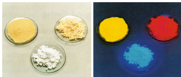
Fig. 10.4 Examples of different types of fluorescent powder as seen under white light ( left ) and under ultraviolet radiation ( right )
