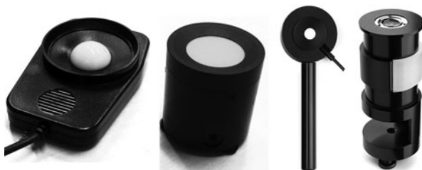
Fig. 14.8 Example of photocell housings with protective layer that together provide cosine correction, and (on the right ) an adapter for the measurement of semi-cylindrical illuminance
