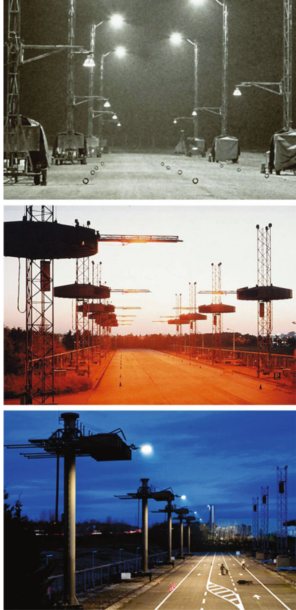
Fig. 3.20 Philips' open-air road-lighting laboratories—from first to third generation. The third generation is today's laboratory in France. (Photo: Pierre Crouzet)
