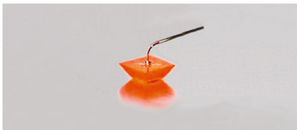
Fig. 10.19 An example of a specifically-shaped LED chip that improves the light-extraction efficiency
