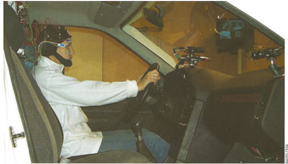
Fig. 3.32 Driving simulator used by Muzet (2003) allowing EEGs to be recorded during simulated (night) drives. Photograph CI2N
