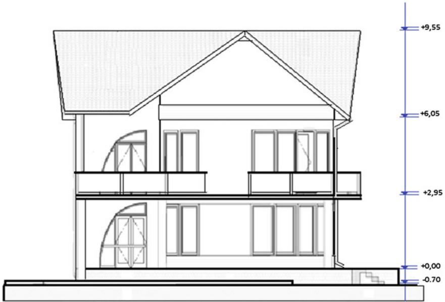
Fig. 2 Frontal view of the building (South facade)
