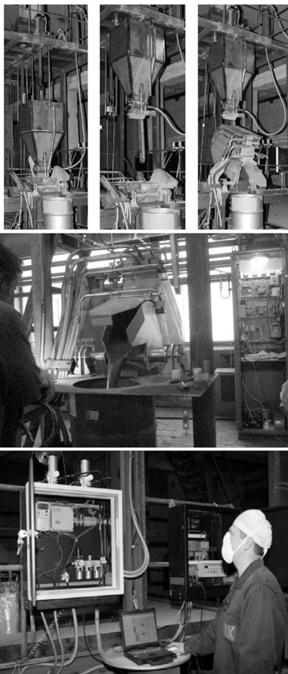
Fig. 2.6 Cementation pilot facility with pulse mixer
