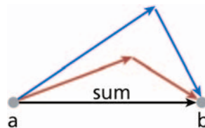
Fig. 22. Knowing the sum of two vectors cannot directly be used to find out which two vectors were added together. There is an infinite number of pairs of vectors that can yield the same sum.
