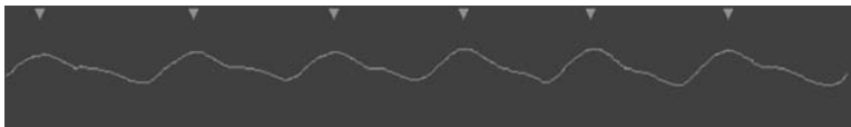
Fig. 3. Signal from the peripheral pulse, with demonstration of triggering with each pulse cycle.
